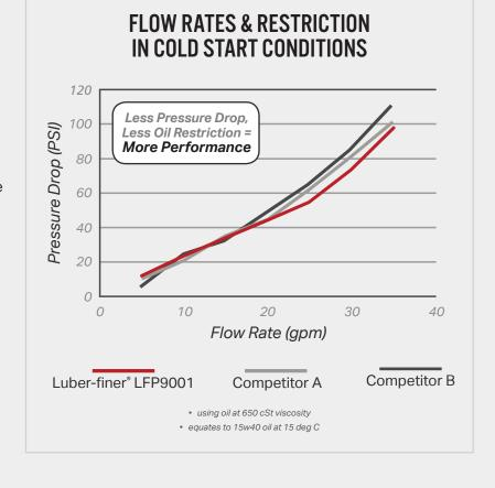
\*At 25 gallons per minute flow rate using ISO4548-1 in-house testing vs competitive filters
