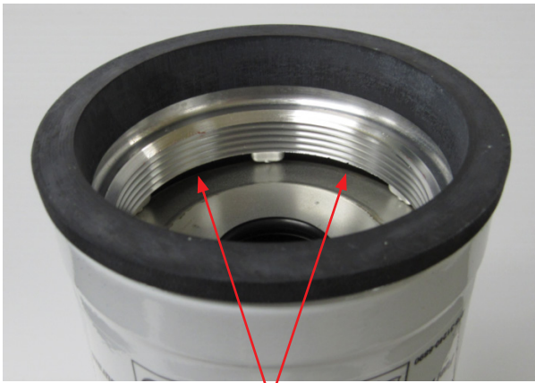
Fuel flow between the tabs
