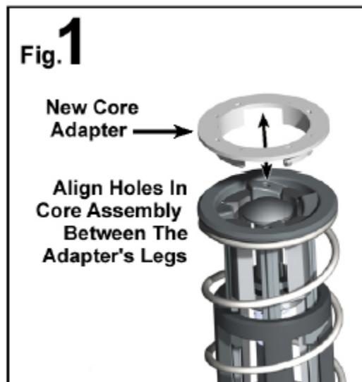
4. With core adapter in position, (see fig 2), press core adapter firmly to snap in place. (see fig. 3)
