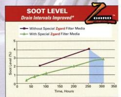
Test conducted in the field with a well-known fleet, whose recommended field replacement was: 4% soot oil or 300 hours. With Zgard, the soot level remained at 3% beyond 300 hours.
