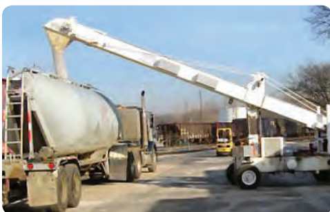
Local sand truck fleets haul the sand from depots to frac sites.
